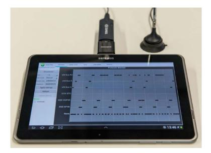
868 MHz Traffic Detective – for cost-efficient and mobile planning and troubleshooting in wireless networks. © Fraunhofer IIS | Picture in color and print quality: www.iis.fraunhofer.de/pr
